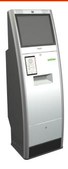
The electronic console **ETR3** consists of an industrial PC with touch screen, dual card reader, biometric identification device, printer, voice communication system and camera. The equipment is installed in a robust steel enclosure with internal heating and temperature monitoring system. This ensures functionality at low temperatures.
