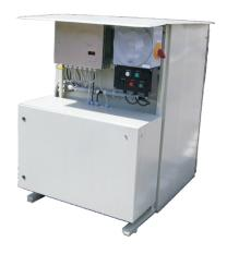
EVA Container is suitable for dosing of additive or color agent into light fuels. It is designed for outside installation in explosive hazardous area. The equipment is designed as an autonomuous skid that includes all necessary components like storage barrel, gear pump, pressure regullation valve, EVA5 injection unit and accessories.
